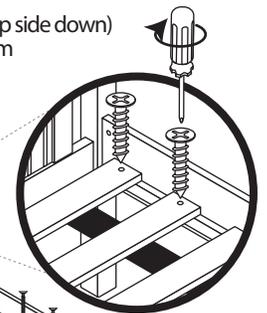
Finally, secure the slats to the side ledges with 30 mm slat screws using a Phillips head screwdriver.
