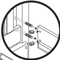
To attach the end boards to the side rails, insert the barrel nuts into the holes in the side rails.
